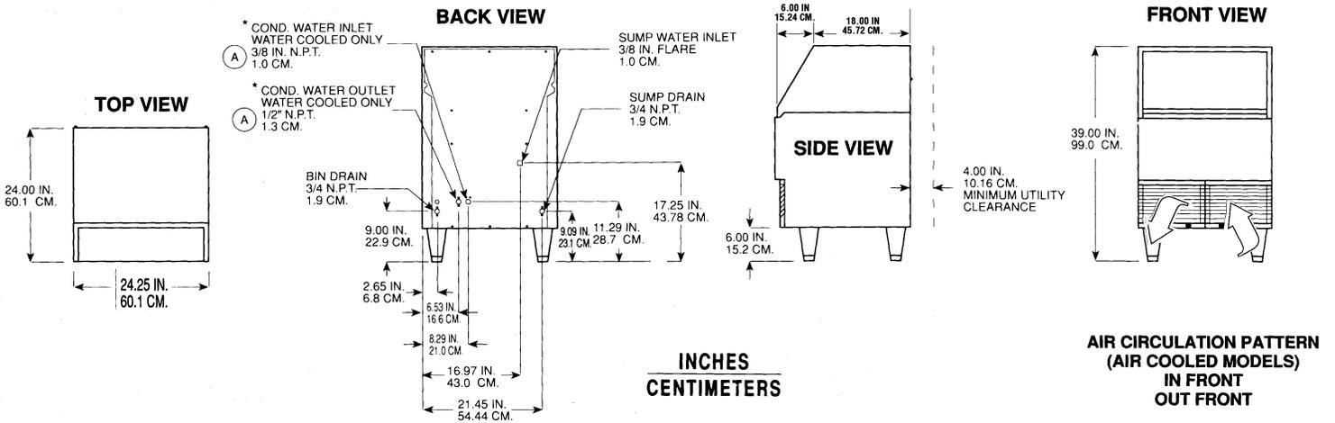
INSTALLATION NOTE: Allow 6" minimum space at left side and back for ventilation and utility connections.
